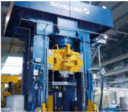
Hydraulic ring blank press with 30,000 kN press force.
