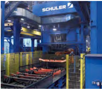
Screw press with direct drive PZS 900f for manufacturing heavy forged parts.
