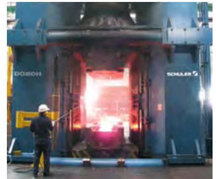
Counterblow hammer with a rated capacity of 800 kJ.
