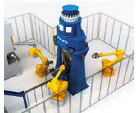
The hammer line is automated with three robots for optimum processes.
