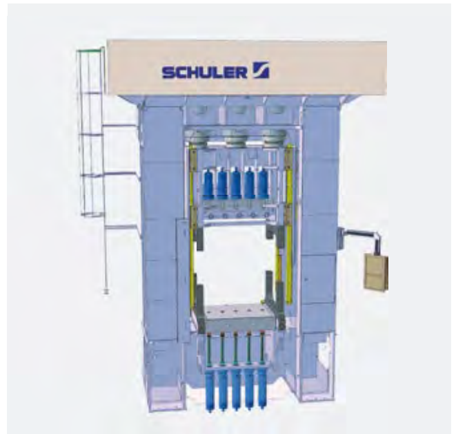
Layout of a multi-station hydraulic cold extrusion press.
