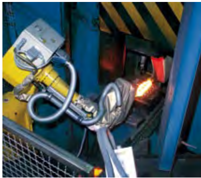
Part handling and forging performed by two robots.
