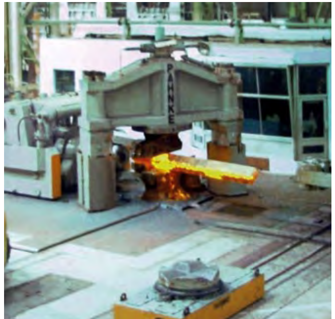
Hydraulic open die forging press with two manipulators.
