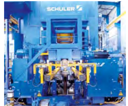
NC-transfer and die space area.
