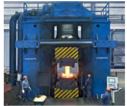
Pneumatic counterblow hammer with a rated capacity of 800 kJ.
