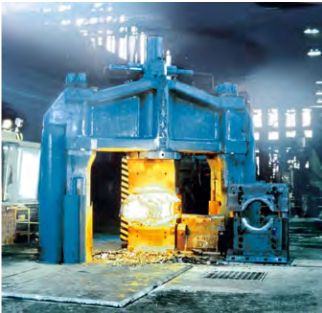
Open Die forging press in underfloor MHFU design.
