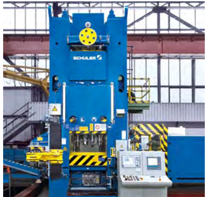
Knuckle joint press with 6,300 kN press force.
