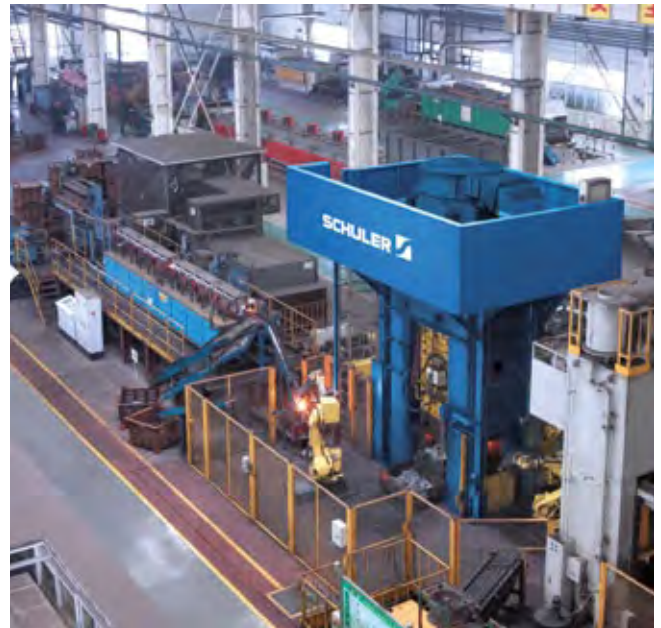
Screw press type PSH 4.450f for manufacturing parts of chain driven earth-moving machinery.
