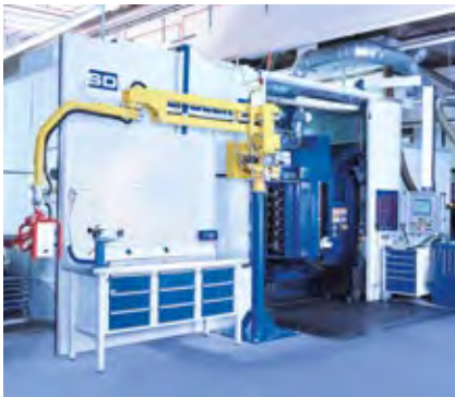
FormMaster with pneumatically supported die change system.
