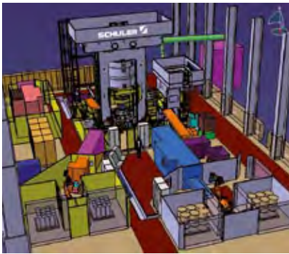
Forging line for manufacturing aluminum wheels.
