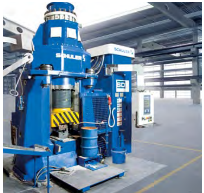
First linear hammer with ServoDirect technology.
