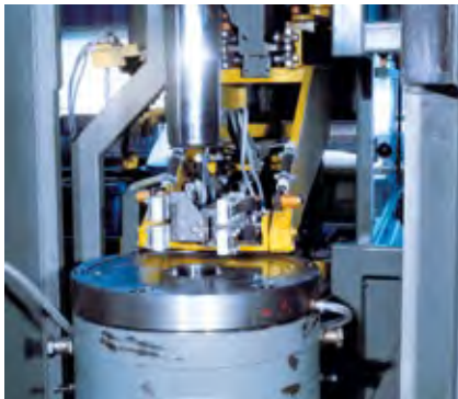
Manipulators transferring the blank from the parts conveyor into the die.
