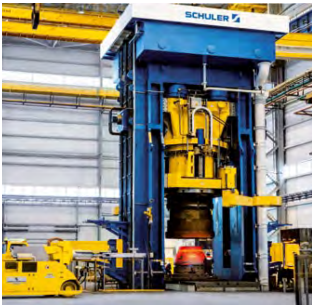
Hydraulic forging press with 140,000 kN press force.
