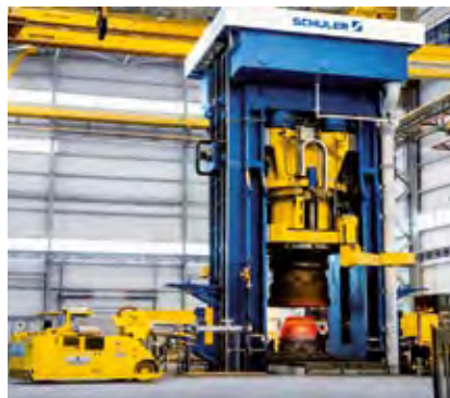
Hydraulic dual forging press with 2 \times 140,000 kN press force.
