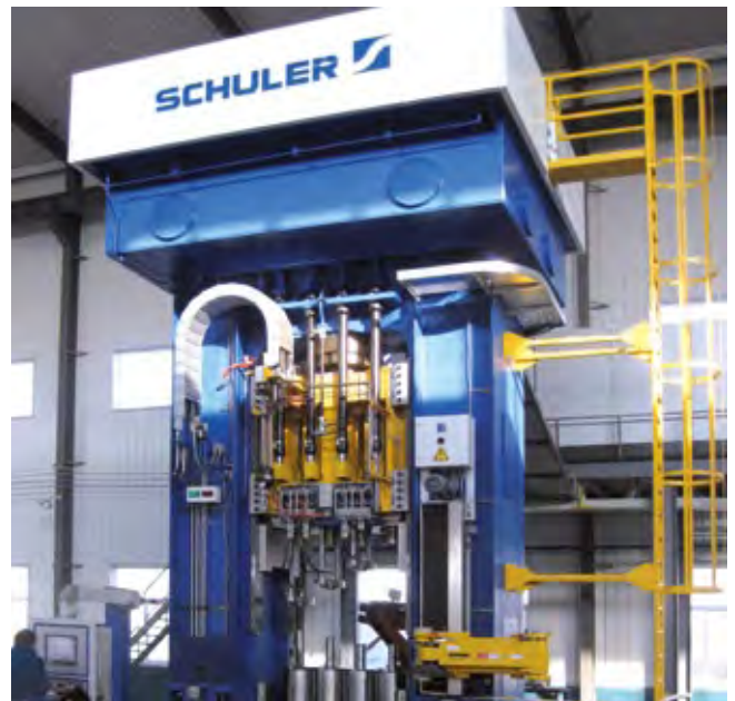
Multi-station closed die forging press with 6,300 kN press force.
