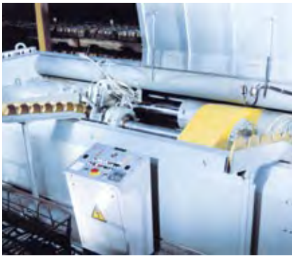
Blanks and cups are processed on the same machine without any return stroke.
