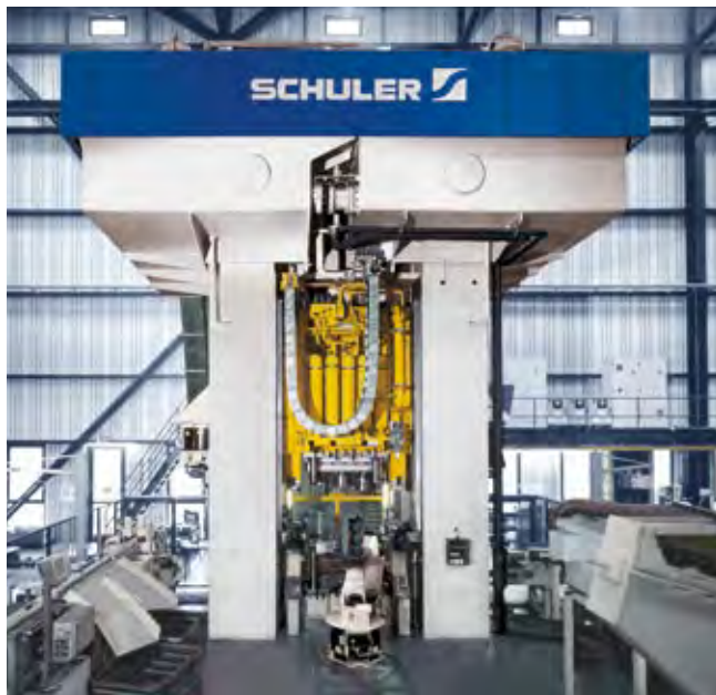
Multi-station hydraulic cold extrusion press with 25,000 kN press force.
