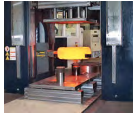
Forging of a ring with symmetrical fiber course.
