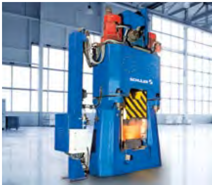
Down stroking hammer with oil hydraulic drive.
