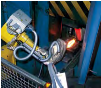
Parts transport and forging using two robots.
