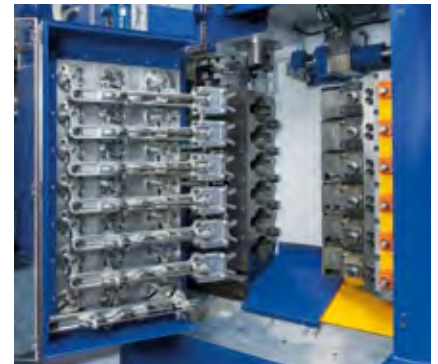
Transfer system and die installation space for 6 forming stations.
