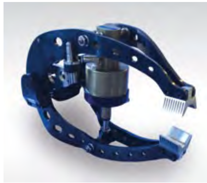
The patented special gripper prevents vibration couplings during hammer forging.
