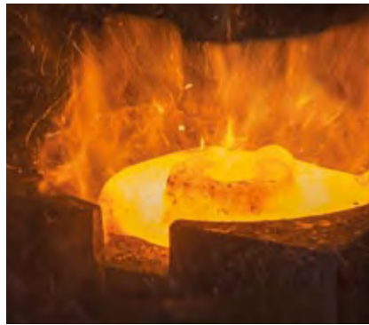
Precision forging with the linear hammer.
