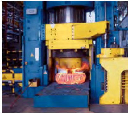
Hydraulic ring blank press with 40,000 kN press force.
