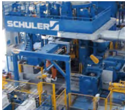
Screw press PZS900 automated with suspended robots.
