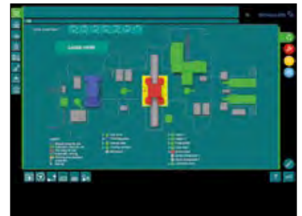
Forge Control System for monitoring the complete forging line.
