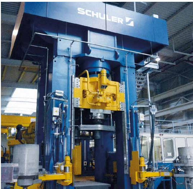
Hydraulic press for forging ring blanks (MH-3000).
