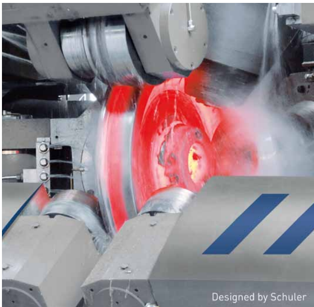
Rolling a freight car wheel on the new Schuler wheel roller.
